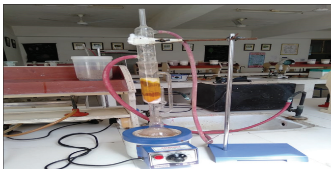
Figure 4: Soxhlet assembly in pharmacognosy department during extraction.
